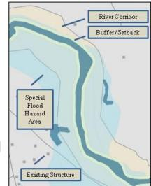
been mapped by approximate methods. Base flood elevations are shown at selected intervals on maps of Special Flood Hazard Areas that are determined by detailed methods. Please note, where Floodways have been determined they may be shown on separate maps.
